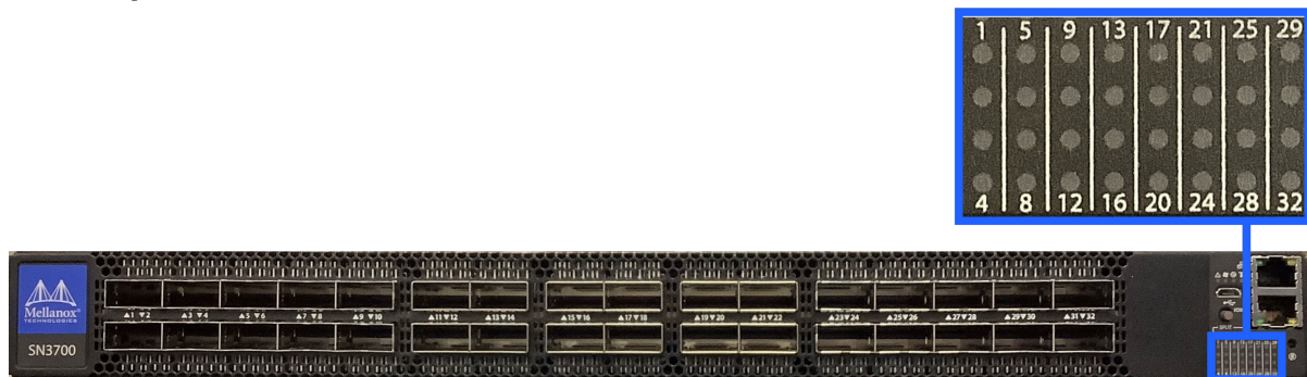
Figure 95. Switch port LEDs of an MTM 5149-S05 switch
