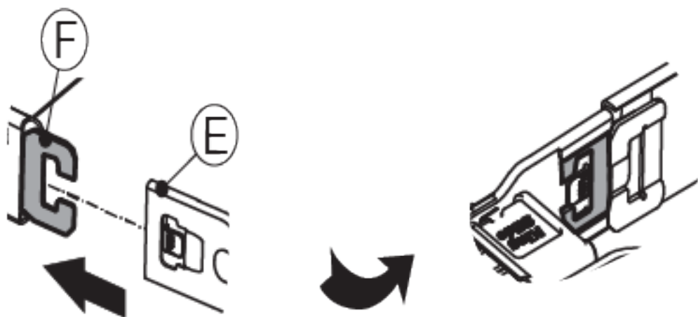
Figure 45. Installing CMA body connector (E) on the left CMA body rail
