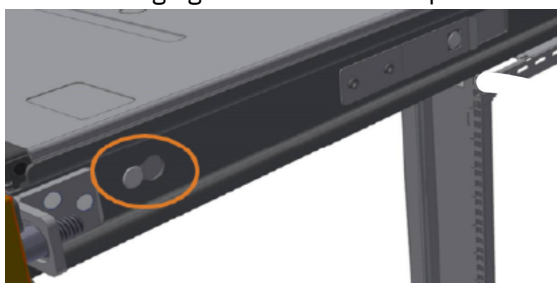
Figure 72. The 5149-N64 switch and rails alignment
