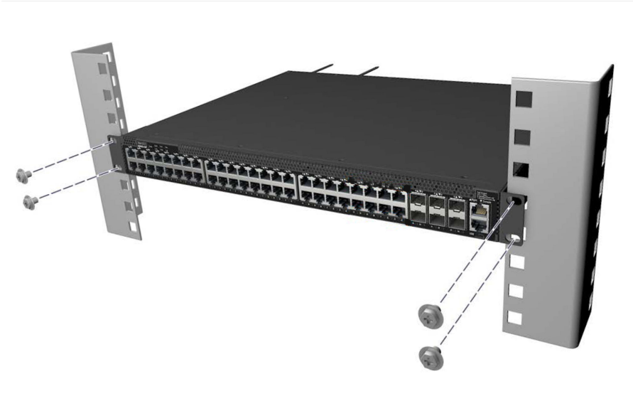
Figure 137. Securing the MTM 5149-S54 switch to the rack
