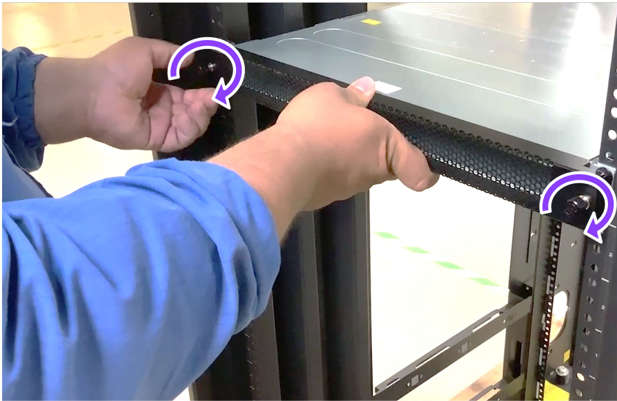
Figure 111. Securing the air duct top
