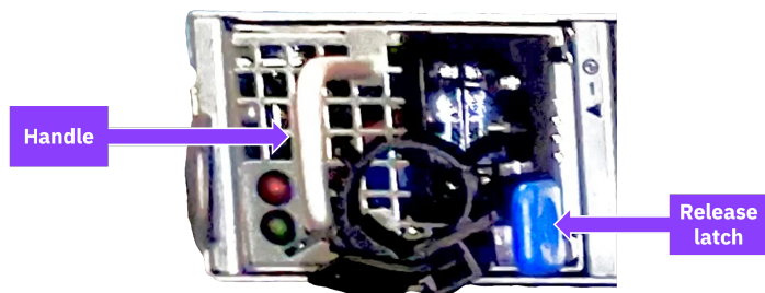
Figure 114. Locating the release latch and handle of a PSU
