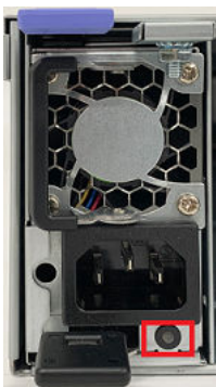
Figure 50. IBM Storage Scale System 3500 power module status LED
