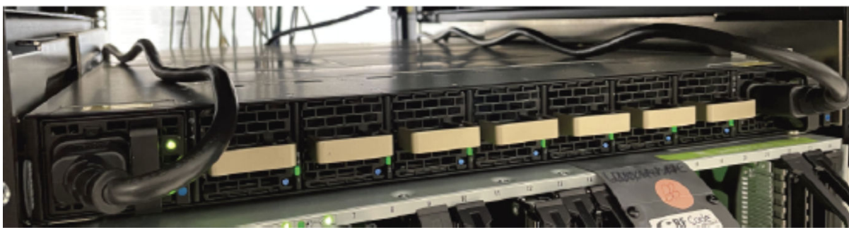
Figure 57. PSUs view of the MTM 5149-N64 switch
