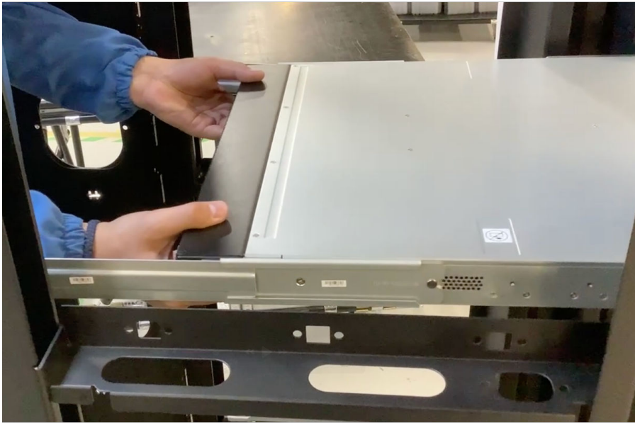
Figure 106. Inserting the rack mounting blades in the rack mounting rails
