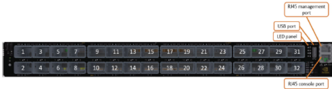
Figure 64. Port view of the 5149-N64 switch
