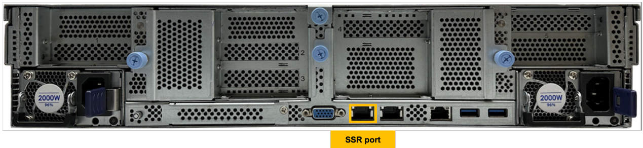
Figure 15. SSR access port in the Utility Node
