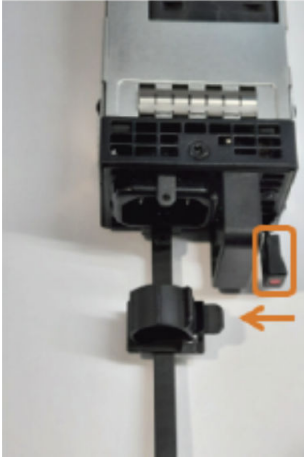
Figure 85. Releasing latch while pulling the handle
