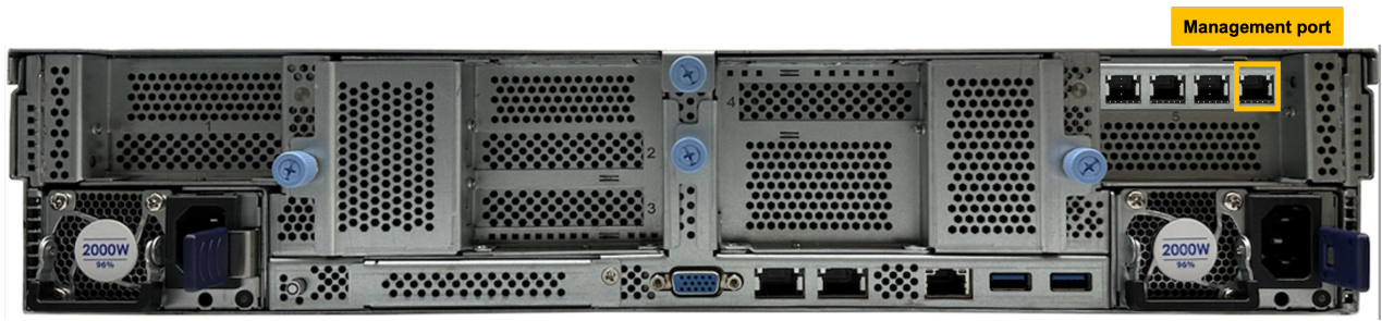
Figure 16. Management port in the Utility Node
