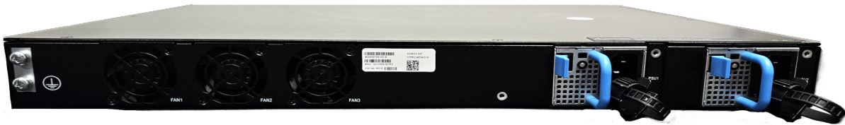
Figure 118. PSUs view of the MTM 5149-S54 switch
